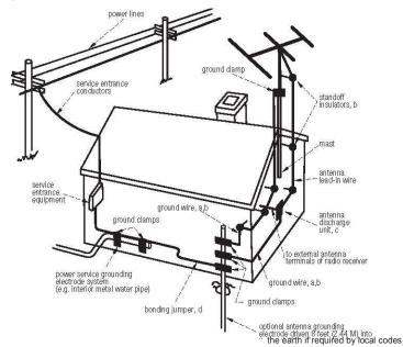
NOTE TO CATV SYSTEM INSTALLER This reminder is provided to call the CATV system installer's attention to Article 82022 of the National Electrical Code that provides guidelines for proper grounding and, in particular, specifies that the cable ground shall be connected to the grounding system of the building, as close to the point of cable entry as practical.
